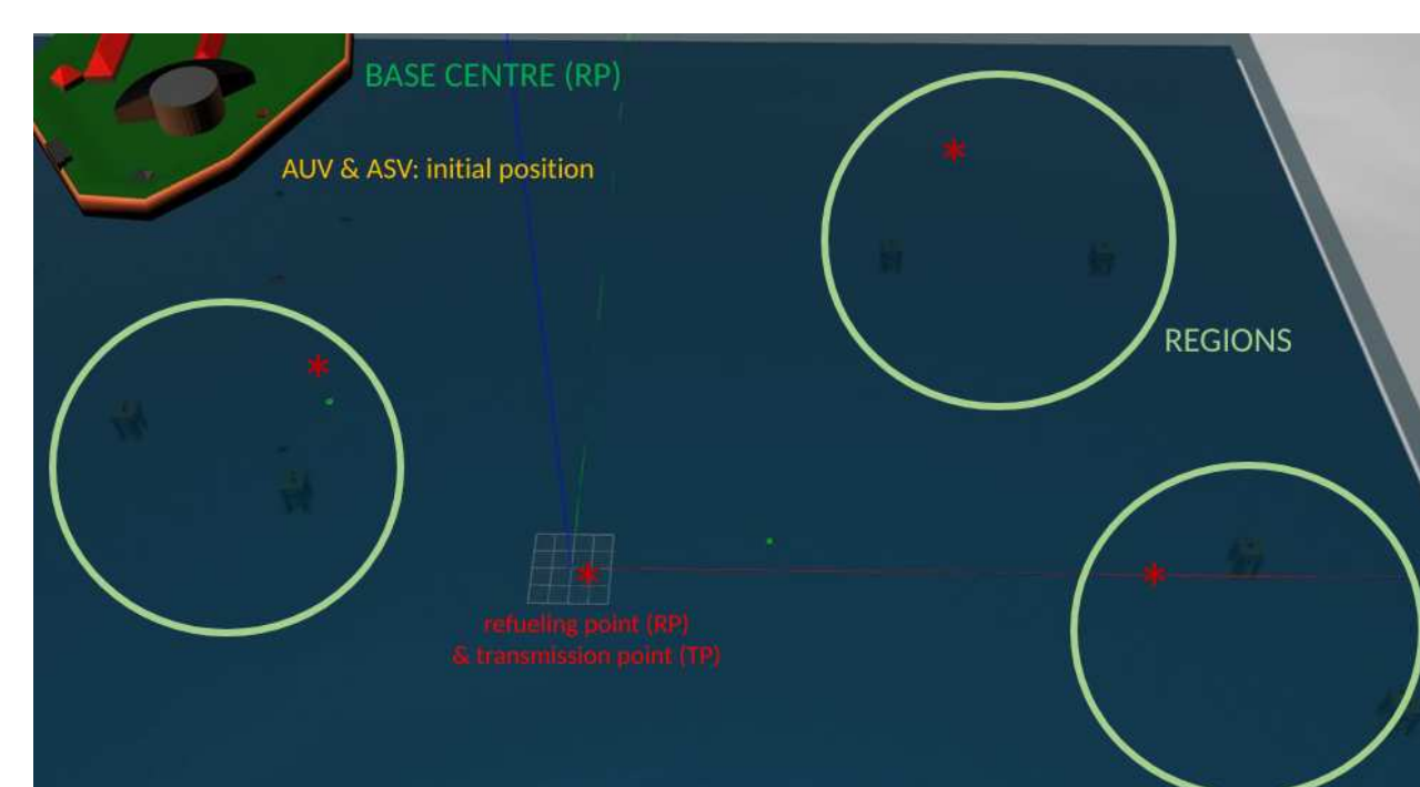
Figure 1: A depiction of the domain which presents the initial position of surface and underwater robots, the docking point (DP) and transmission centre (TC).
